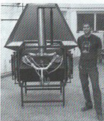
Fig 4 Double-ended recuperated glory hole with integral hood by Wet Dog Glass, LLC
